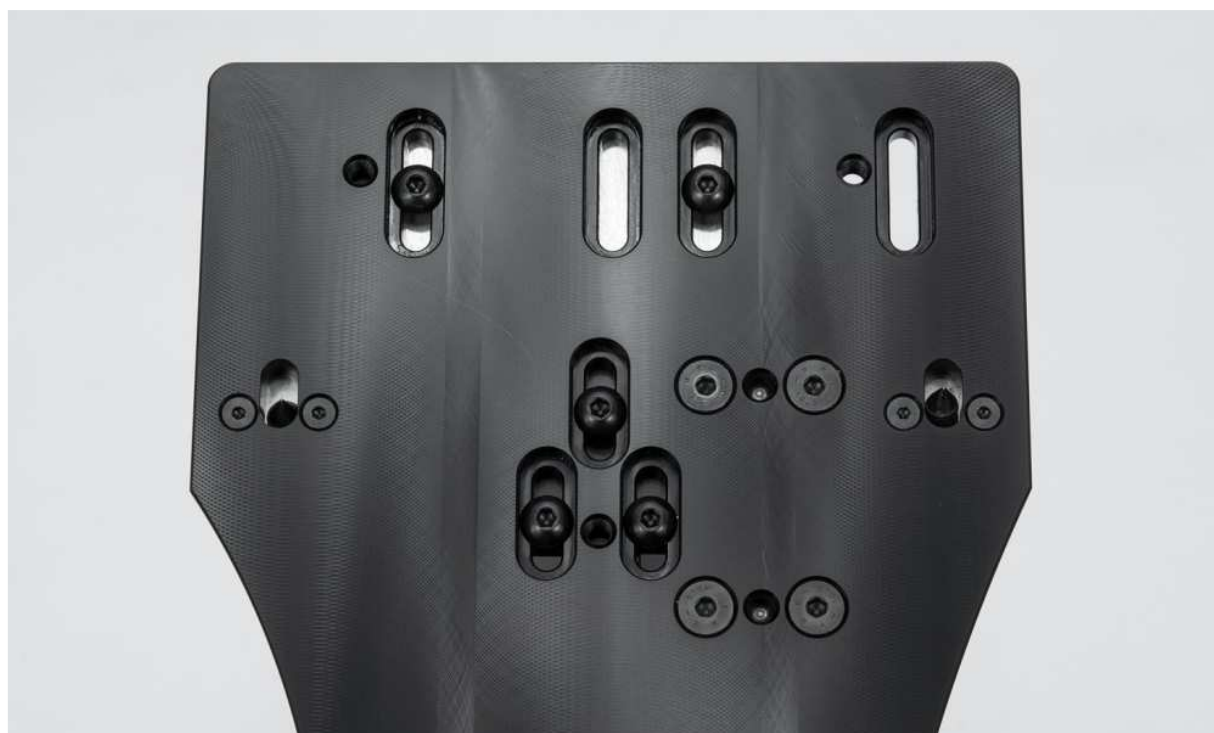
Fot.5.3.2 Clamping device - configuration 2xSINGLE and SINGLE - screw spacing – bottom view
